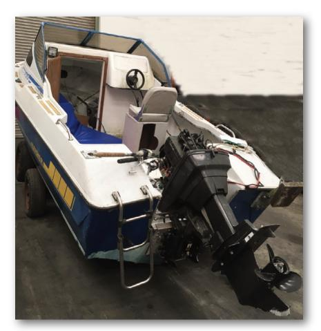
Photograph No.1 - The boat from astern - note height of transom in way of outboard.
